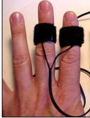
Figure 3. Example configuration for GSR electrodes. Modified from Michael Gasperi's website ( http://www.extremenxt.com/gsr.jpg ).
